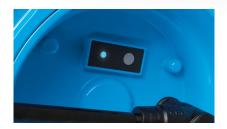
Press the button next to the LED which will illuminate blue for two seconds followed by two short white flashes to confirm connection to the LCD or Gateway.
